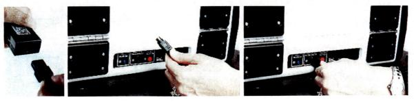
4. Plug the flat end of the USB printer cable from the ballot printer into the back of the Verity Print, with the notch facing up. ▼
