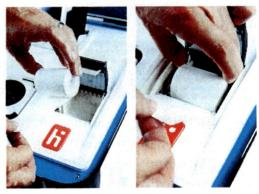
4. Close the printer cover. The paper must extend out from underneath the front edge of the cover. The white button can be used to advance the paper.
