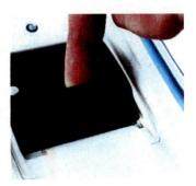
To replace paper: Place the new paper roll into the printer as shown. Paper must roll up from the bottom. ▶
