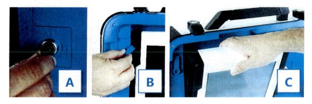
7. Seat the tablet in the cradle (A), tilt it back (B), and lock it in place (C). ▼
